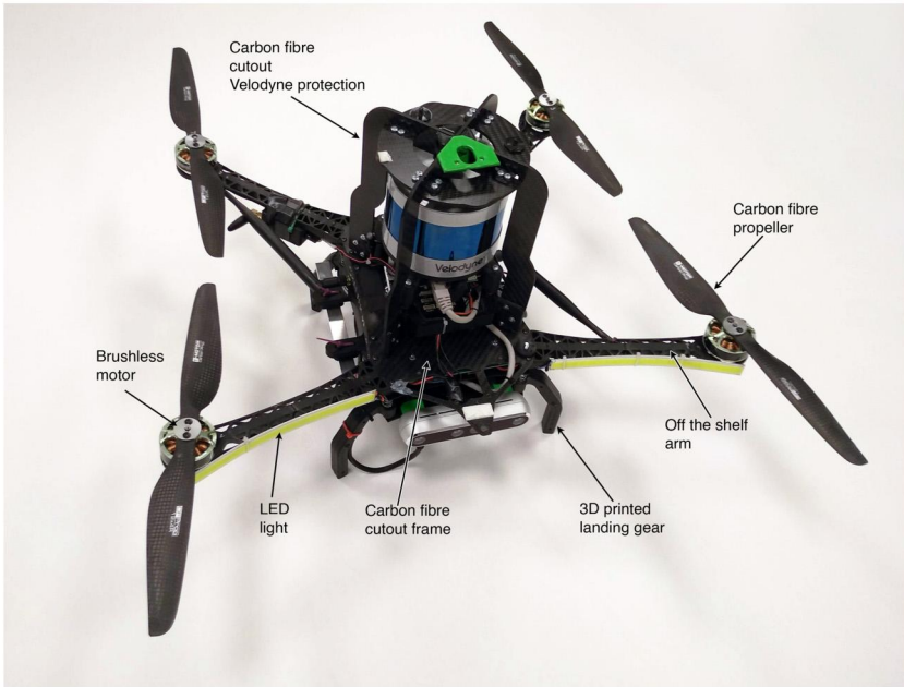
FIGURE 2.9 “Shafter” was constructed using a combination of carbon fiber sheet cutouts and commercially available arms.
