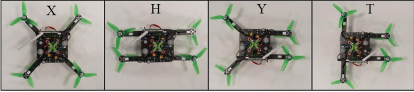
FIGURE 8.9 Different formations X , H , Y , and T based on re-configurable ARW's arms position.
