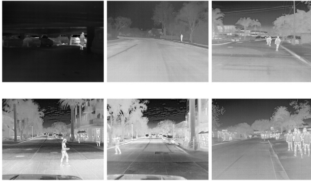
FIGURE 10.10 Examples of the extracted images from the FLIR ADAS dataset in the case of a human detection. The images are extracted while the camera approaches to the human.
