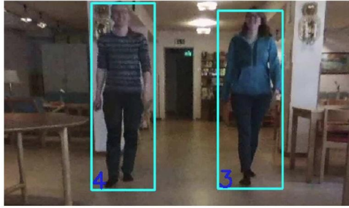
FIGURE 5.5 An example of YOLO detecting two people in an indoor environment and the Hungarian algorithm tracking them.
