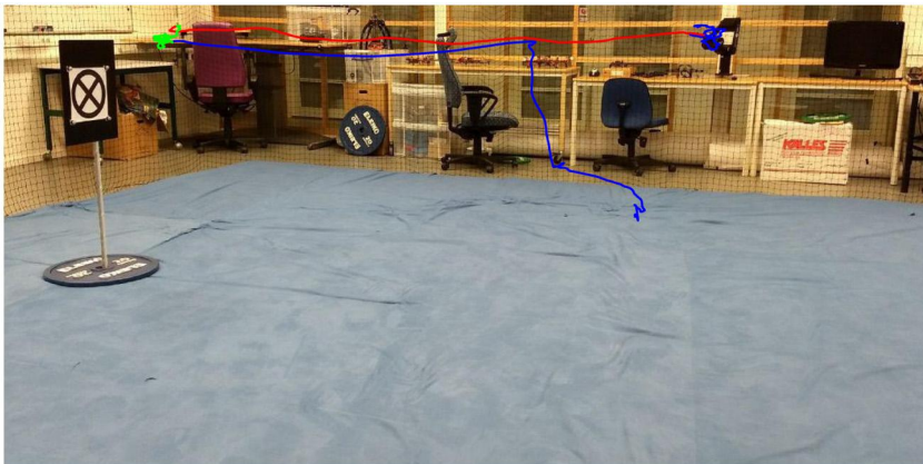
FIGURE 9.11 MAV actual trajectory derived from the experimental trials of the stereo-based guidance. Case 2: the end-effector reaches the target. The developed guidance system contributes to the task with the red (gray in print) and green (light gray) part of the overall trajectory. The red part is followed after the extraction of the centroid, while in the green part the robotic platform is hovering. The blue (dark gray) parts of the trajectory consist of the initialization (hovering on a fixed position) and termination phases (landing) of the experiment.
