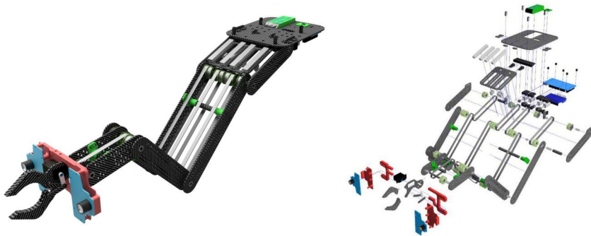
FIGURE 9.5 Left – CAD design of the CARMA manipulator. Right – CARMA parts explosion view.
