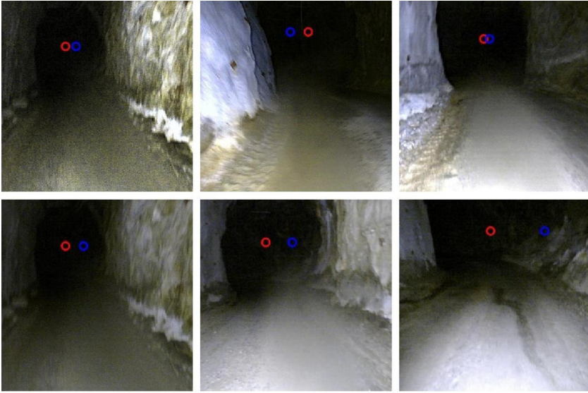
FIGURE 12.27 Comparison of s_x from CNN and centroid extraction method from ARW onboard camera. The CNN estimation is indicated by a blue (dark gray in print) circle, while the centroid extraction method is indicated by a red (lighter gray in print) circle.
