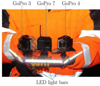
FIGURE 12.18 The triple camera setup for obtaining training data sets for CNN.
