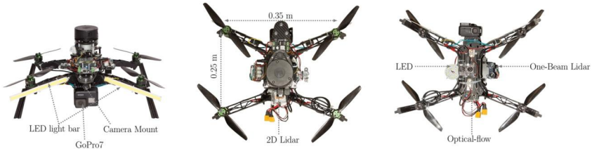
FIGURE 12.7 The developed quadcopter equipped with a forward looking camera, a LED lights, optical flow, 2D lidar, and single beam lidar.
