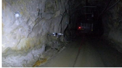
FIGURE 12.29 The ARW navigates close to the wall due to the stand-alone CNN module and the corresponding absence of a potential field module for obstacle avoidance in the Bebop case.
