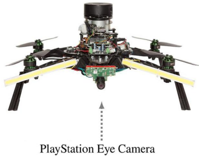
FIGURE 12.17 The ROSflight based platform equipped with PlayStation Eye camera.
