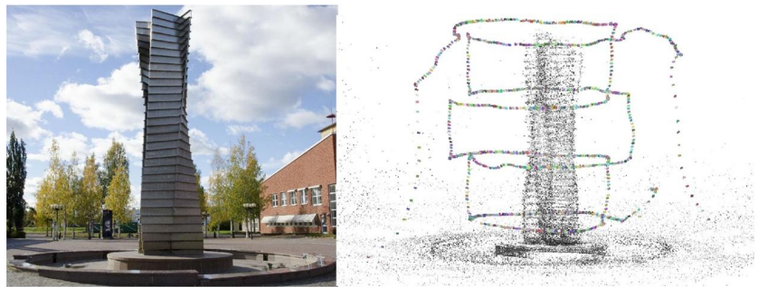
FIGURE 11.19 On the left is the Luleå University's outdoor fountain, and, on the right, the cooperative pointcloud of the structure with estimated flight trajectories.
