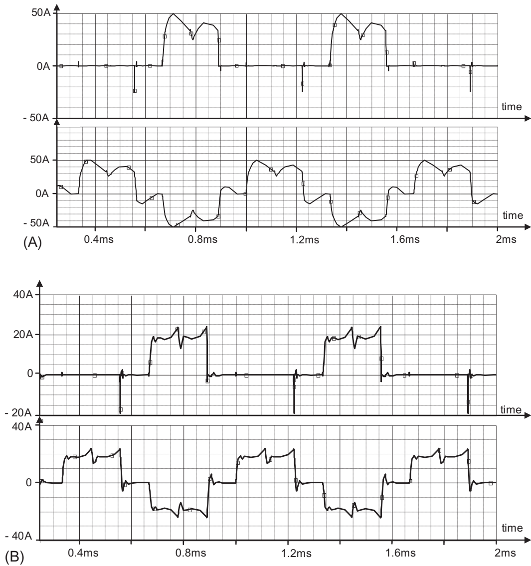
FIG. E1.3.3 (A) MOSFET (upper graph) and motor (lower graph) current for phase angle \theta = 0 degree. (B) MOSFET (upper graph) and motor (lower graph) current for phase angle \theta = 30 degree.
