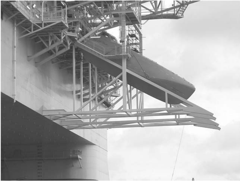
Figure 5.4 Free-fall lifeboat type. The concept of launching of the free-fall lifeboat into the sea uses the force of gravity as an ally and dispenses control through cables and descent mechanisms, which increases the reliability of the operation. The hull is wedge-shape, which allows the transfer of the launch energy at the time of contact with the sea. Photograph courtesy of the supplier norsafe: www.norsafe.com .
