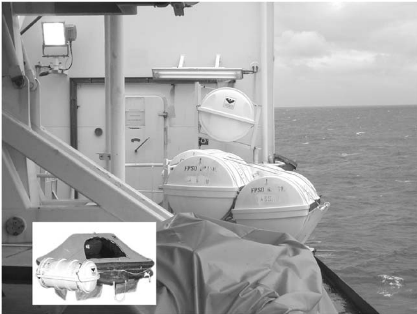
Figure 5.6 Life rafts positioned inside the storage cylinders, ready for launching from the main deck of the offshore rig. The detail view illustrates the appearance of the inflated life raft after being launched into the sea.
