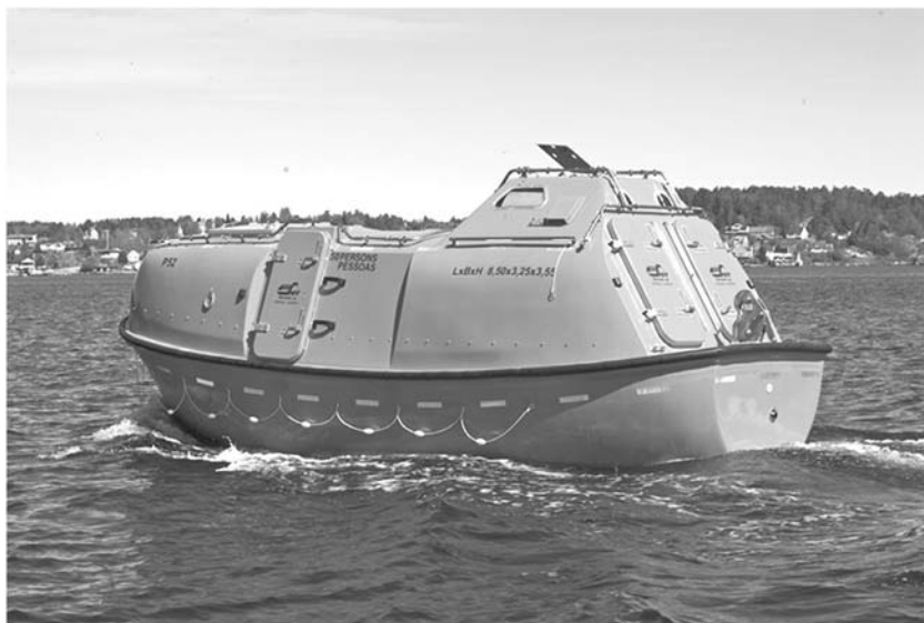
Figure 5.3 Conventional lifeboat (rescue vessel). The concept of launching of the lifeboat into the sea includes support by steel cables during the descent operation. The hull is not wedge-shaped and does not withstand the impacts of a free fall. Photograph courtesy of the supplier norsafe: www.norsafe.com .
