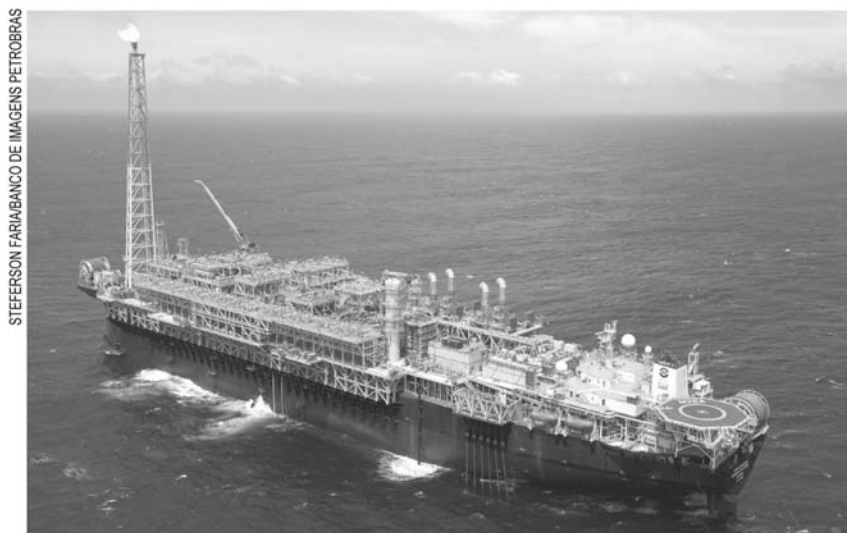
Figure 3.8 FPSO rig. FPSO, Floating production, storage, and offloading rig system.
