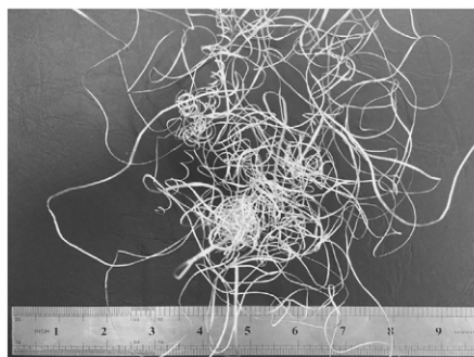
(A) Tool without chip breaker
