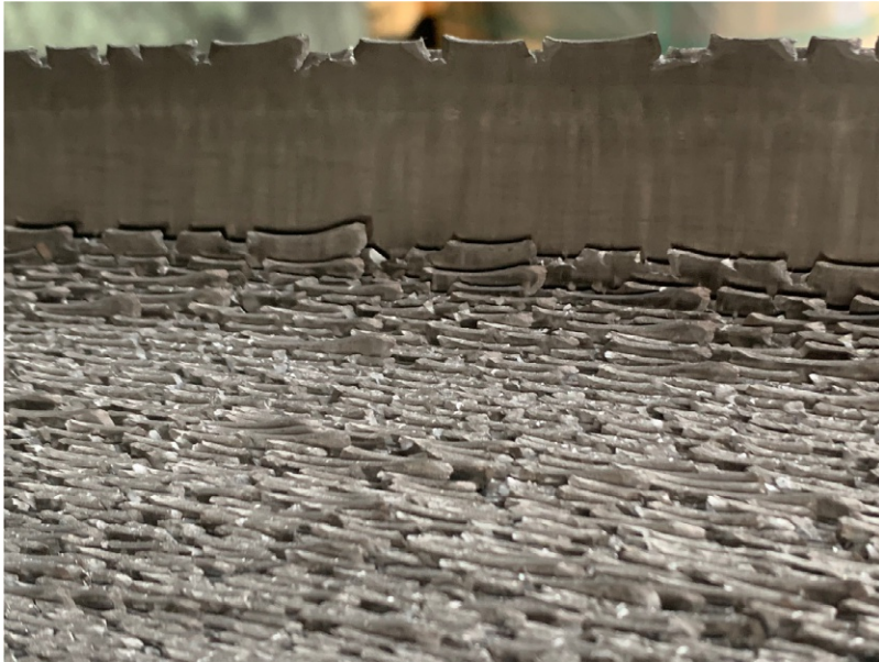
Edge cracks in a cold rolled 5754 Al sheet (thickness 1 mm).
