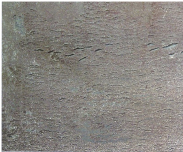
Fig. 12.13 Surface transversal cracks in a strip after hot rolling. (Magnification is not known.)
