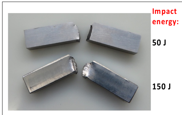
Charpy V-notch specimens broken after impact testing.
