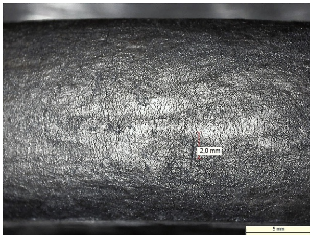
Fig. 11.14 Hot upsetting at 1150°C of a resulfurized steel containing bismuth, with the formation of very few surface cracks by barreling (Oliosio, 2021).
