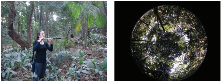
Figure 5.9. LAI measurements with the plant canopy analyzer and the hemispherical pictures technique at Trianon Park, 2012. (Photos: P. Shinzato)
