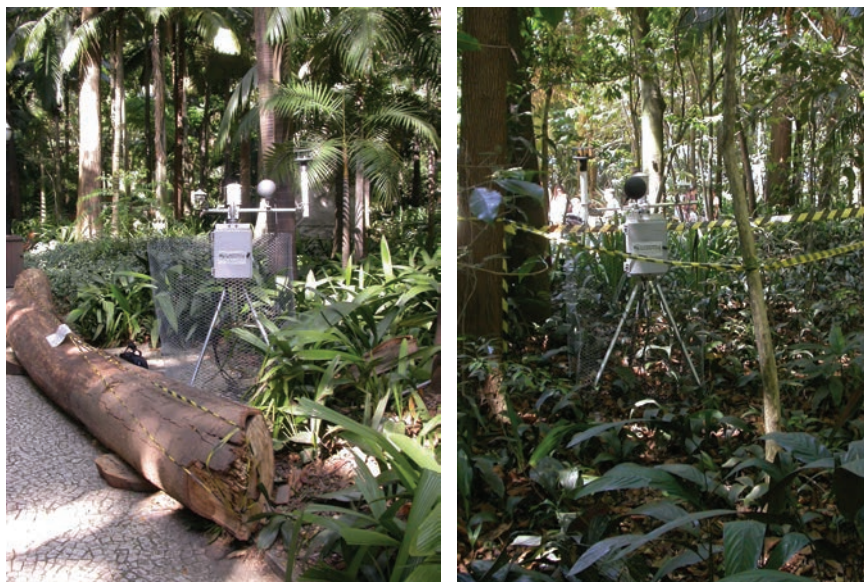
Figure 5.10. Meteorological stations at points 1 and 2 inside Trianon Park, set up at 1.5 m above ground level, in November 2013. (Photos: P. Shinzato)
