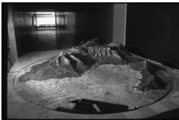
Figure 4.6. Topographical model of Table Mountain in the wind tunnel. (Source: Dr Adam Goliger)
