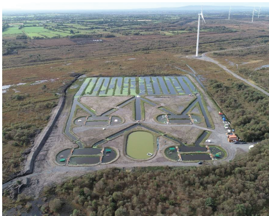
Fig. 10.14. Aerial view of the Oasis Fish Farm in Ireland. The water storage reservoir is located bottom center of the site with the four fishponds spaced around it, each separated into four sections. Water from the fishponds flow through channels on the outer sides of the site to enter either end of the duckweed treatment pond. The treatment pond is divided into two sections, both discharging treated water at the center, which flows back to the fishponds via the centrally located channels. Water is moved around the site by numerous surface paddle wheels that also oxygenate the water, using electricity powered by the adjacent wind farm. Image by Gary McCoy and reproduced with permission of Bord Iascaigh Mhara.
