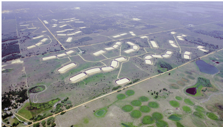
Fig. 8.3. Rapid infiltration basins used for groundwater recharge of wastewater that has received advanced treatment at Orlando, Florida. Reproduced with permission from the US Geological Survey.
